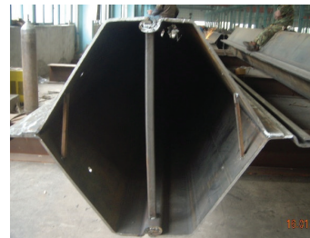
Box King Piles (fabricated out of 2 CRZ Piles & 1 Cold Formed U Pile)
