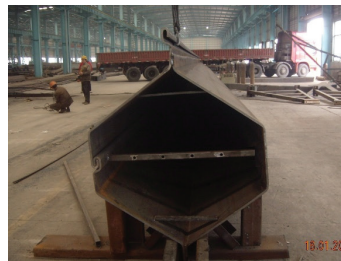
Box King Piles (fabricated out of 2 CRZ Piles)
