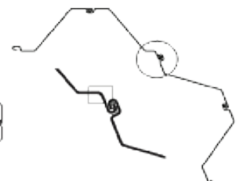
OPTION 3 Cold Form bending of flange
